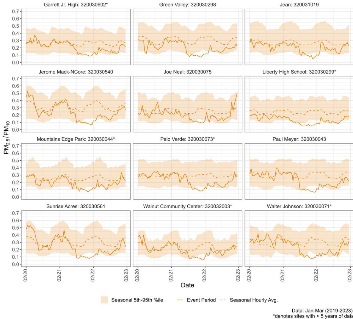
Figure 3.3-6. Ratio of PM_{2.5}/PM_{10} concentrations at the Garret Jr. High, Green Valley, Jean, Jerome Mack, Joe Neal, Liberty High School, Mountains Edge Park, Palo Verde, Paul Meyer, Sunrise Acres, Walnut Community Center, and Walter Johnson sites before, during, and after the February 21, 2023, PM_{10} event. The five-year average PM_{2.5}/PM_{10} diurnal ratio is displayed as a dotted line, and the 5th to 95th percentile range is shown as a shaded ribbon. The average and 5th to 95th percentile ratio is calculated across January-March of 2019-2023.
